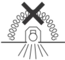
3. Luminaires not suitable for covering with thermally insulating material.
