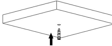
3. Fix the suspended ceiling plate on the ceiling.
